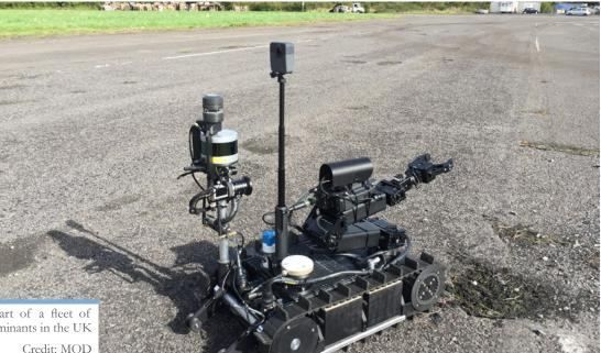
This remote controlled robot is apart of a fleet of drones that test for chemical contaminants in the UK
